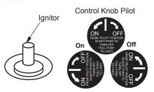
Figure 19 - Ignitor and Control Knob
